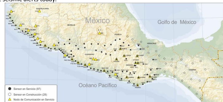
Figure 1. The solid black circles represent the distribution of sensing stations used in the Mexican Seismic Alert System. (from Espinosa-Aranda et al., 2014).
